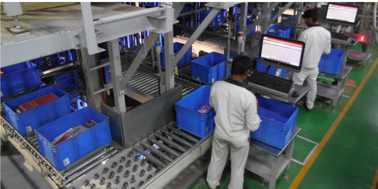
Goods-to-person fulfilment improves the efficiency and accuracy of the picking process. It is also easily scalable and uses a smaller footprint than person-to-goods fulfilment.
