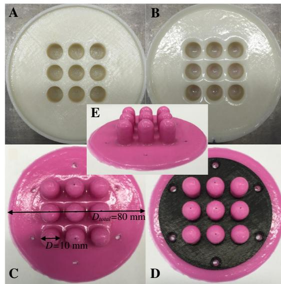
Figure 2. Fabrication of PapillArray prototype. ABS mould A) before and B) after acetone vapour bath; C) silicone prototype, top view; D) prototype with mounting support; E) silicone prototype, side view.
