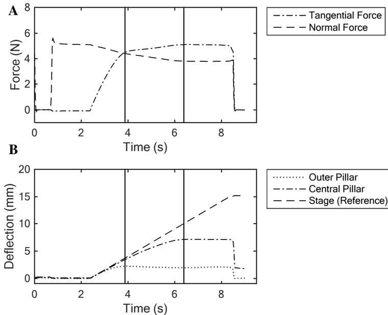
Figure 7. A) Force and B) pillar deflection data used for testing pillar slip behaviour – high friction surface (acrylic treated with dried soap), 5 N normal force level, 4<sup>th</sup> repetition. Moment of slip is indicated by solid vertical line – left-most vertical line for outer pillar, right-most vertical line for central pillar.
