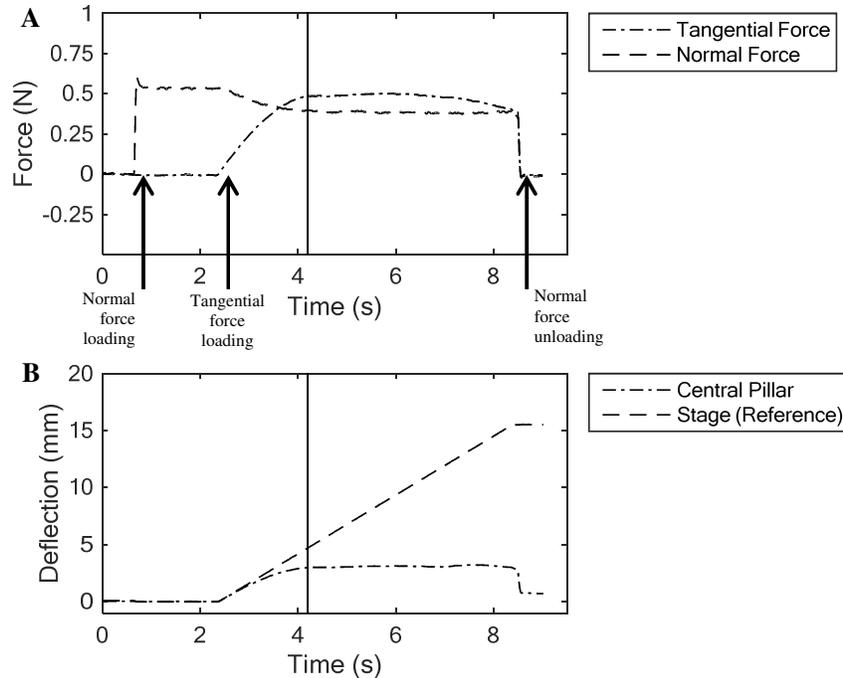
Figure 6. A) Force and B) pillar deflection data used for friction calculation – High friction surface, after 5 N test. Moment of slip of central pillar is indicated by solid vertical line.
