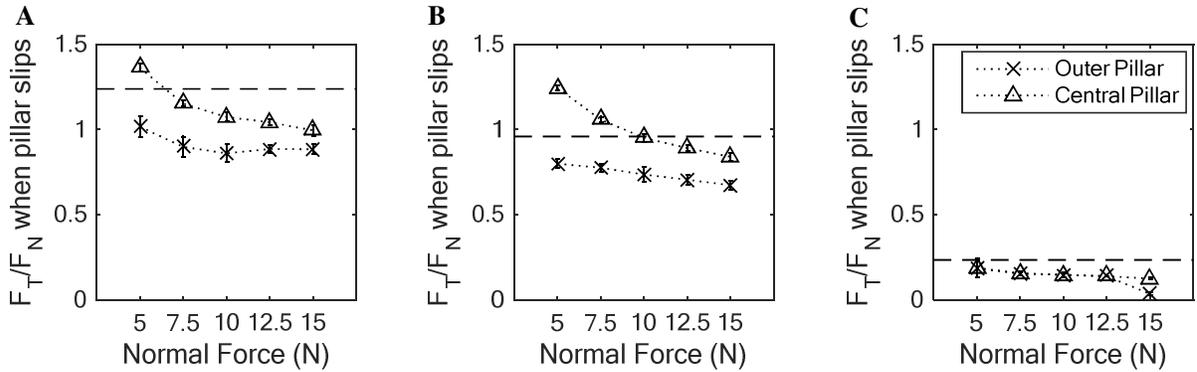
Figure 8. Tangential-to-normal force ratio at which each pillar slips at each normal force level for the A) high, B) base, and C) low friction surfaces. Markers are the mean values and error bars extend to  $\pm$  SD. Dashed horizontal line indicates  $\mu_s$  measured at 0.5 N normal force.
