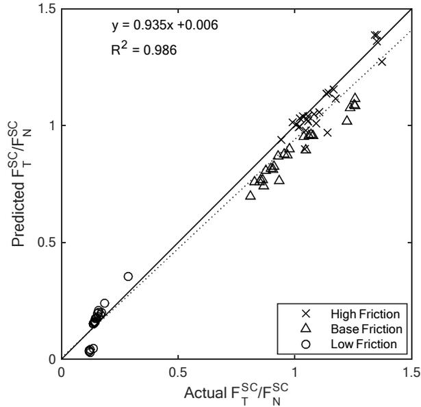
Figure 10. Actual and predicted ratio  $F_T^{SC}/F_N^{SC} = F_T^{SO}/(F_N^{SO} - kd)$  with line of best fit, equation and  $R^2$  value.
