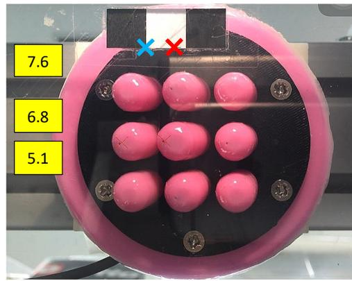
Figure 4. A single frame of video captured during the testing procedure. The red cross is the original position of the marker; the blue cross is the current position of the marker which moves with the acrylic plate. The values highlighted in yellow are the deflections (mm) of the marker (top), the central pillar (middle), and the outer pillar to the left of the central pillar (bottom).
