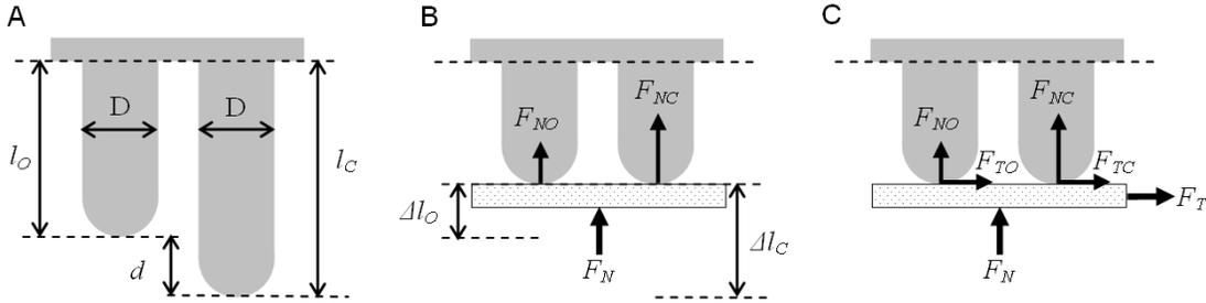
Figure 1. Illustration of a central pillar and outer pillar of a PapillArray sensor with nine pillars (one central pillar surrounded by eight outer pillars). Each pillar has a diameter  $D$ , and the central and outer pillars have uncompressed heights  $l_C$  and  $l_O$ , respectively. The sensor is shown when A) it is uncompressed, B) it is compressed with a flat surface, and C) the surface is sheared.
