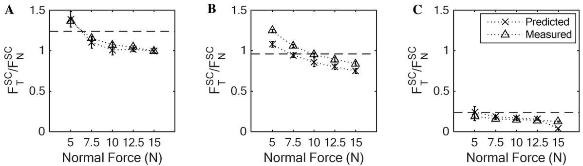
Figure 9. Actual and predicted  $F_T^{SC}/F_N^{SC}$  for each normal force level for the A) high, B) base, and C) low friction surfaces. Markers are the mean values and error bars extend to  $\pm$  SD. Dashed horizontal line indicates  $\mu_s$  measured at 0.5 N normal force.
