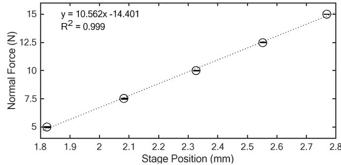
Figure 5. Calculating the spring constant of the silicone. Stage position for each normal force with line of best fit, equation and  $R^2$  value. Markers are the mean values and error bars extend to  $\pm$  SD.
