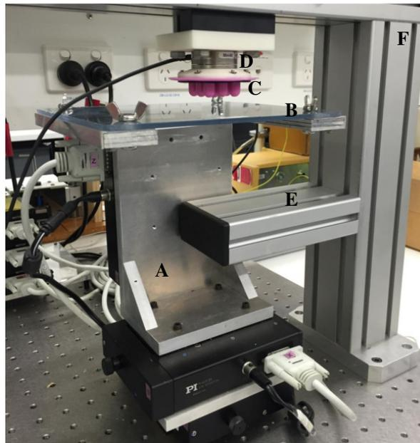
Figure 3. Test rig. A) XYZ-stage, B) acrylic surface, C) PapillArray prototype, D) 3D force/torque sensor, E) platform for video capture, and F) support frame.
