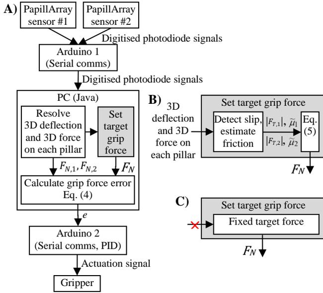
Figure 3. A) Block diagram of gripper system, setting the target grip force in the B) dynamic grip force control strategy, and C) fixed grip force control strategy which does not use any tangential force or friction information from the PapillArray sensor (only normal force from the PapillArray is used).
