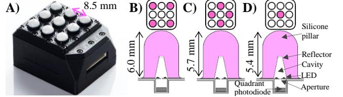
Figure 1. A) Photograph of a PapillArray sensor, and dimensions of B) corner (shortest) pillars C) middle-height pillars, and D) central (tallest) pillar. For all pillars, the pillar outer diameter is 6 mm, the diameter of the base of the conical cavity is 4 mm, the reflector diameter is 2 mm, the aperture diameter is 0.8 mm, the reflector to aperture distance is 3.5 mm, and distance from the aperture to the top of quadrant photodiode is 2.0 mm.
