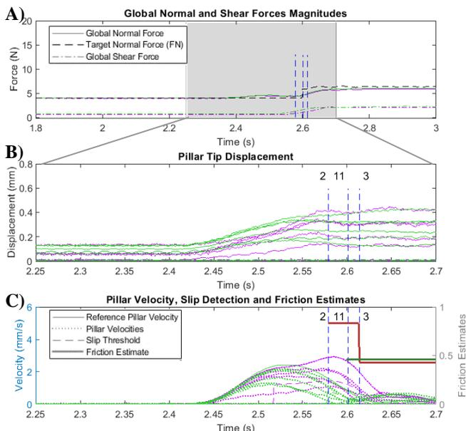
Figure 6. Example of sensor output during lifting task with dynamic grip-force control. Light custom-made object (431 g) with cardboard surface (high friction). See Fig. 5 caption for other information.
