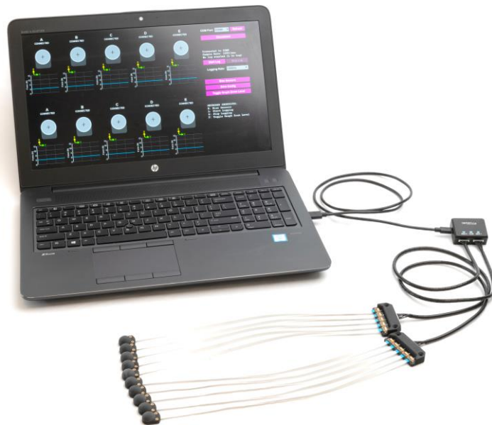
Figure 1.1 – The 3D Force Button Sensor Development Kit (Beta v1.0). Laptop not included.
