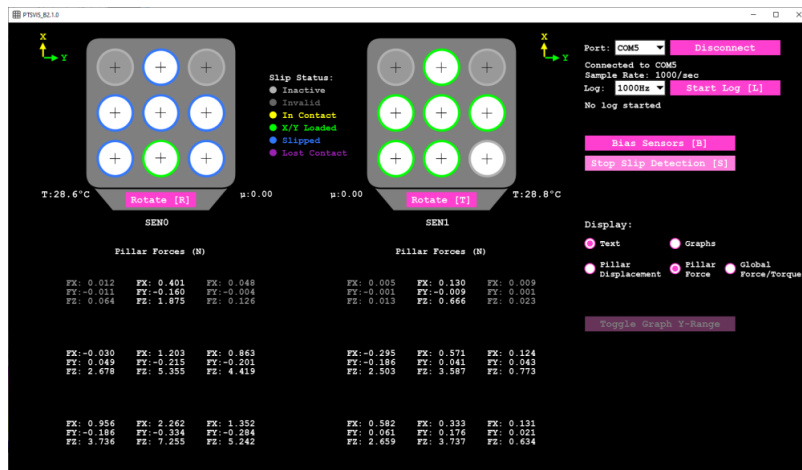
Figure 1.2 – The PapillArray Tactile Sensor Visualisation Software (v2.1).
