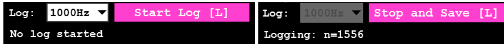
Figure 7.4 – Left: Log file controls before starting a log. Right: Log files control during logging
